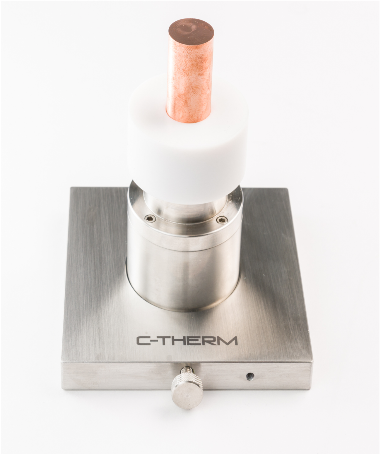
Testing Copper with MTPS
