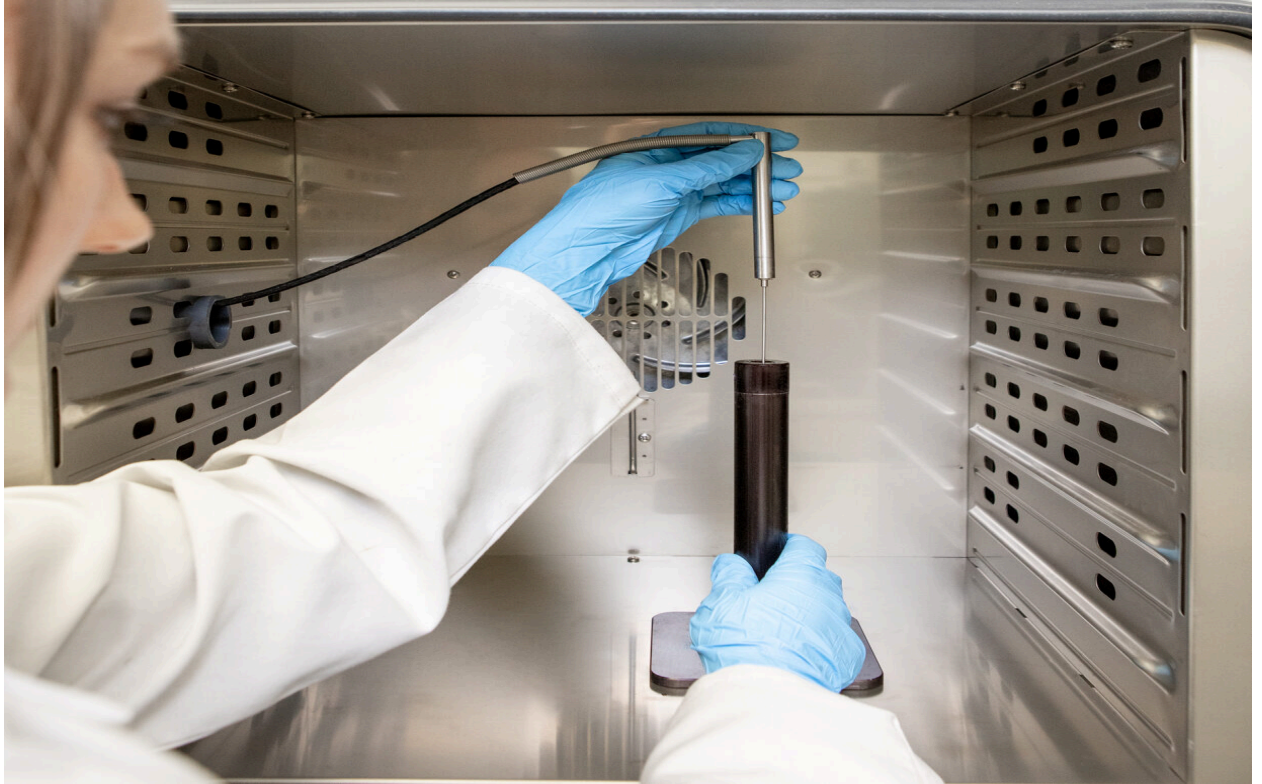
A scientist using the TLS needle probe in a thermal chamber, the probe is being placed into a vial containing the sample powder.
